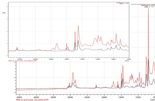
Figure 3: FTIR-ATR absorption spectrum of virgin ABS (black) and recycled post consumer ABS (red)
